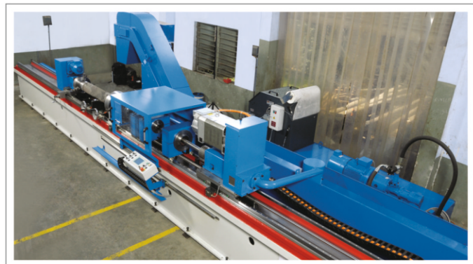
CNC Deep Hole Boring Machine Ø18 to Ø150 mm up to 4500 mm Length
