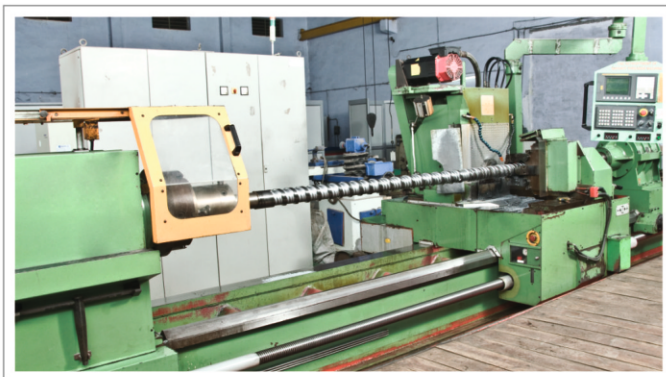
CNC Thread Milling Machine Ø14 to Ø250 mm up to 5000 mm Length
